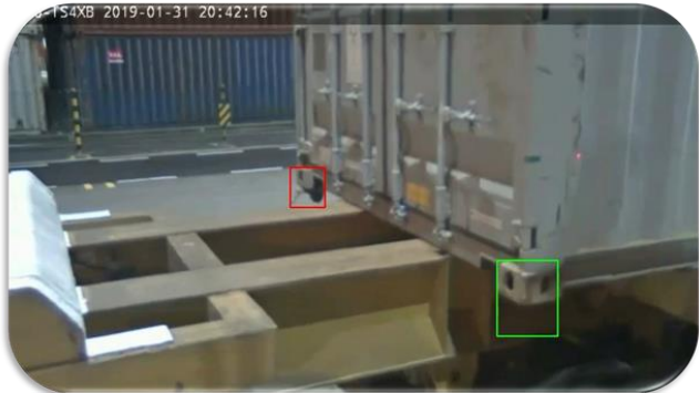
Detection of twistlock (highlighted by red rectangle)
