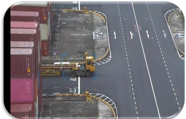
PM failing to stop at stop-line
