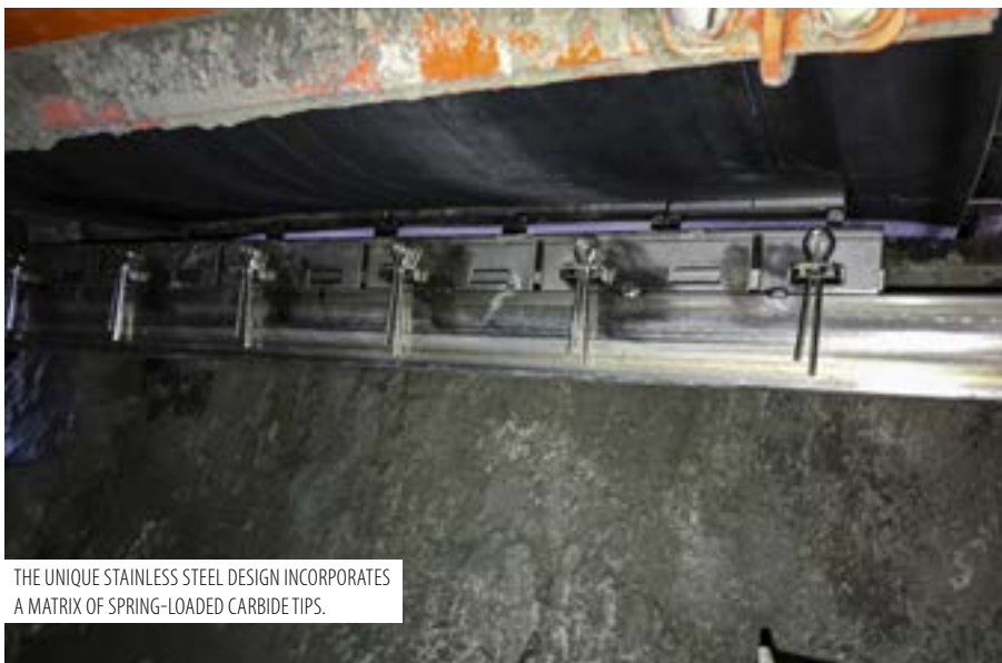
THE NEW SECONDARY BELT CLEANER IS ENGINEERED TO MINIMIZE MAINTENANCE AND CONVEYOR STOPPAGES.
