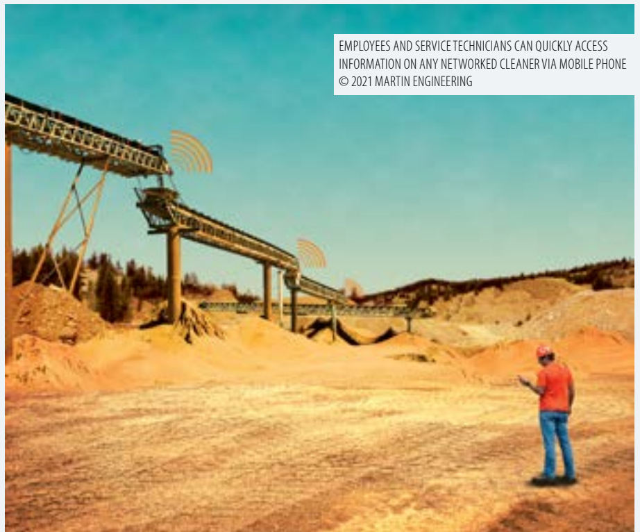
THE N2 PI NOTIFIES SERVICE PERSONNEL WHEN A CLEANER REQUIRES RE-TENSIONING OR REPLACEMENT
