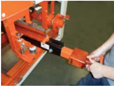
THIS SLIDE-OUT BELT CLEANER IS ENGINEERED TO BE ACCESSED SAFELY AND REPLACED BY A SINGLE WORKER © 2020 MARTIN ENGINEERING
