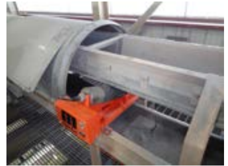
THE UNIQUE BELT CLEANER FORMS A 3-D CURVE BENEATH THE DISCHARGE THAT CONFORMS TO THE PULLEY'S SHAPE © 2020 MARTIN ENGINEERING
