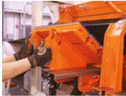
THE TRACK-MOUNTED SYSTEMS CAN BE SERVICED QUICKLY AND SAFELY, WITH NO REACH-IN MAINTENANCE © 2020 MARTIN ENGINEERING
