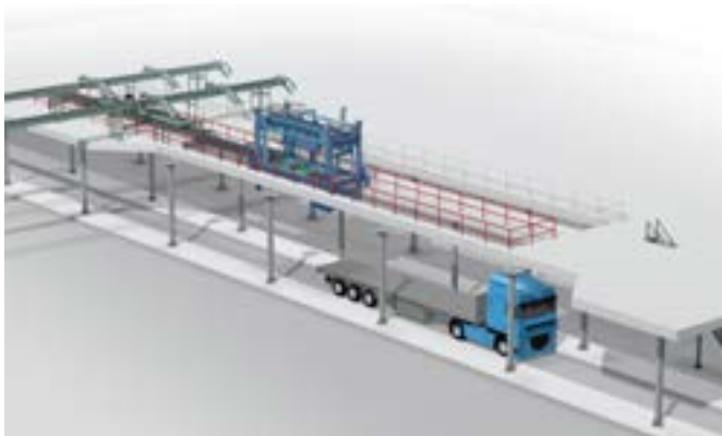
THE TRUCK IS MOVED UNDER THE BEUMER AUTOPAC
