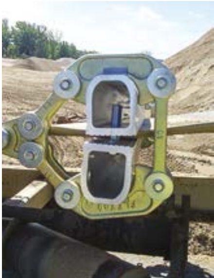
BELT CLAMPS CAN BE AS SMALL AS TWO BARS OR AS LARGE AS A GIANT VICE. © 2020 MARTIN ENGINEERING
