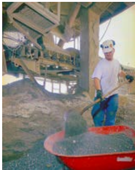
CLEANUP BRINGS WORKERS WITHIN CLOSE PROXIMITY OF A MOVING CONVEYOR. © 2020 MARTIN ENGINEERING
