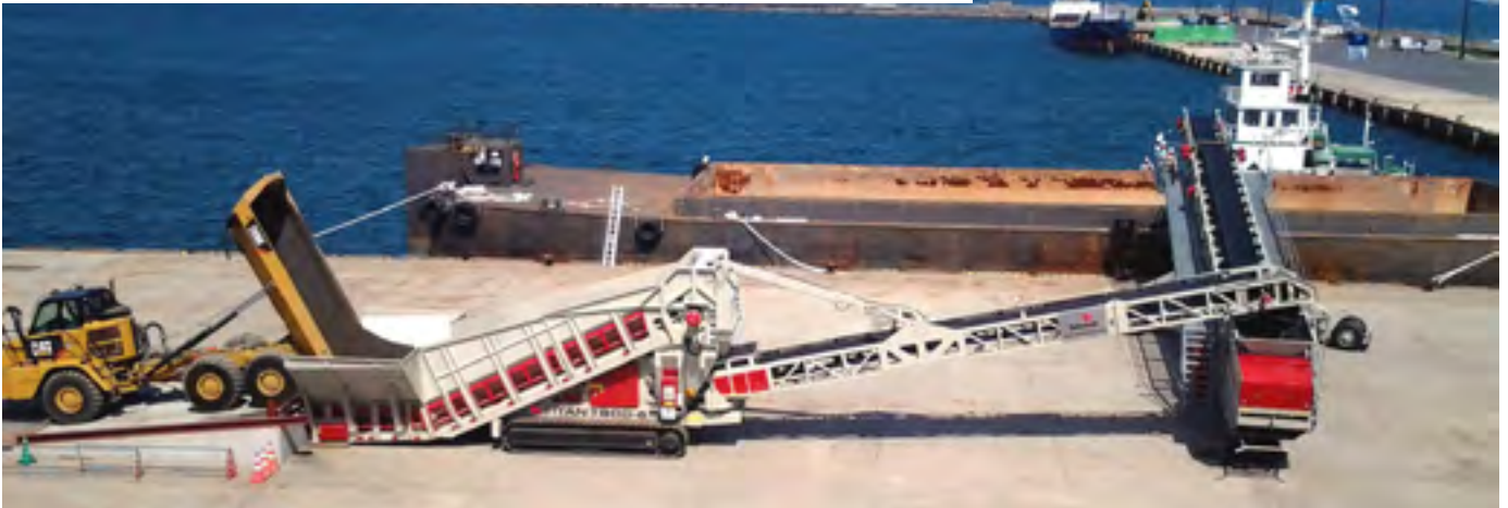
THE TELESTACK TITAN T800-6 AND TS1042 RADIAL TELESCOPIC SHIPLOADER DESIGNED AND MANUFACTURED IN TELESTACK AND EXPORTED TO JAPAN TO BE USED AS PART OF A MULTI-MILLION POUND LAND RECLAMATION PROJECT BY A LARGE POWER UTILITY COMPANY
