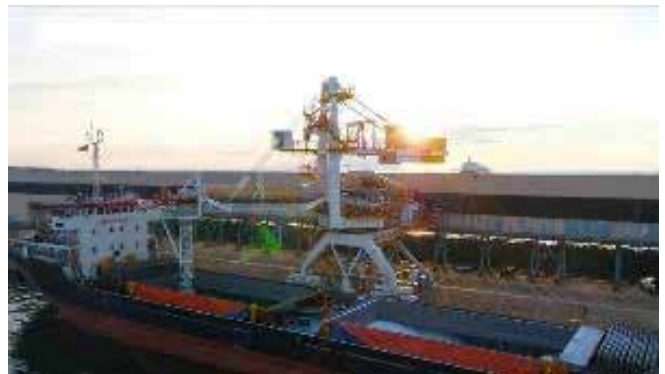
The ship loaders ensure fast and reliable loading of ships in the ports
