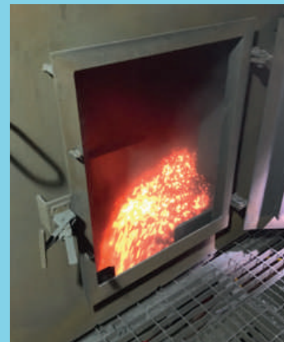
The Aumund steel plate conveyor type KZB-H will transport iron ore pellets at up to 750°C to the cooler. (Photo AUMUND)
