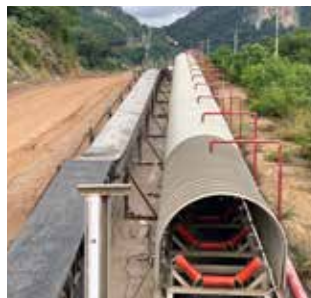
The single belt coils are vulcanised to a long belt next to the conveying system and joint to the old belt. Photo credits: BEUMER Group GmbH & Co. KG
