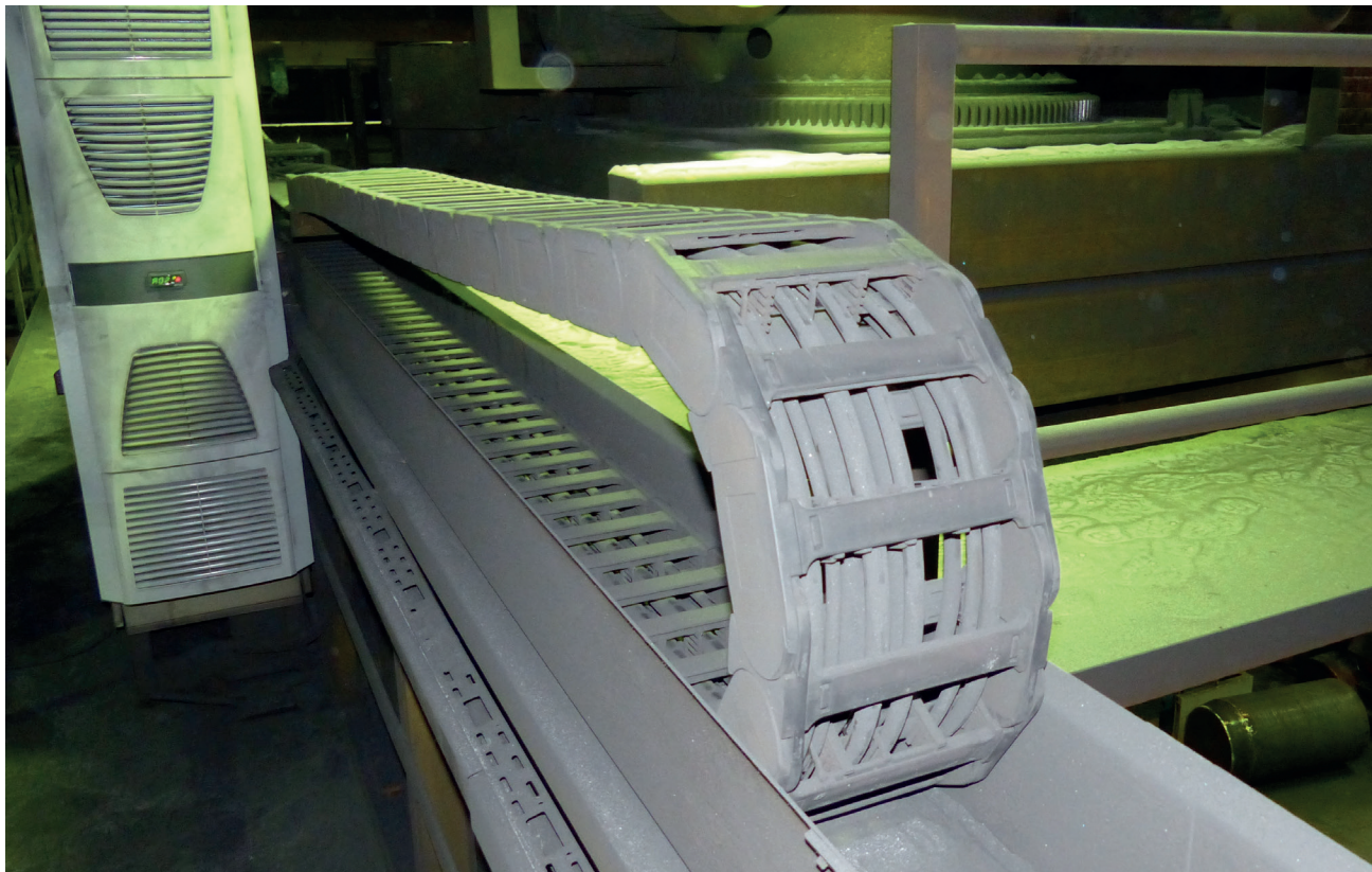
Figure: Energy chains used for long travels in a dirty environment (igus®)
