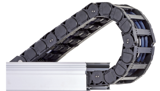
Energy chains are movable protective cages for safely guiding cables and hoses in moving applications. Picture: Source: igus® GmbH
