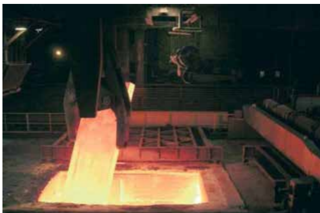
Mechanical claw on a slab crane directly above a furnace (source: igus® GmbH).
