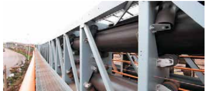
Beumer Group is supplying a 4,150 t/h bi-directional pipe conveyor to the Port of Saguenay. The system will be installed inside an enclosed gallery structure for ease of maintenance during the winter months (© Beumer Group GMBH & Co. Kg)
